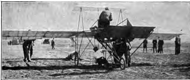
Fig. 49. Curtiss Racing Machine. This is Practically a Monoplane
